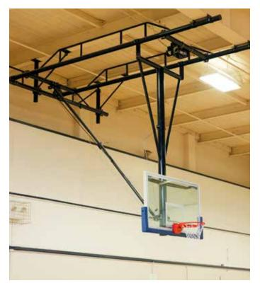
T-frame top is mounted to heavy-duty trolley assemblies that roll on I-beam tracks, allowing the top of the T-frame to roll forward as backstop folds back. This system supports the use of rearfolding backstops at locations closer to walls or other obstructions. Backstops are custom designed so the lateral sway brace intersects the main mast at approximately 54" (1.37 m) above the goal and 18" (46 cm) above the backboard; to ensure maximum rigidity.
